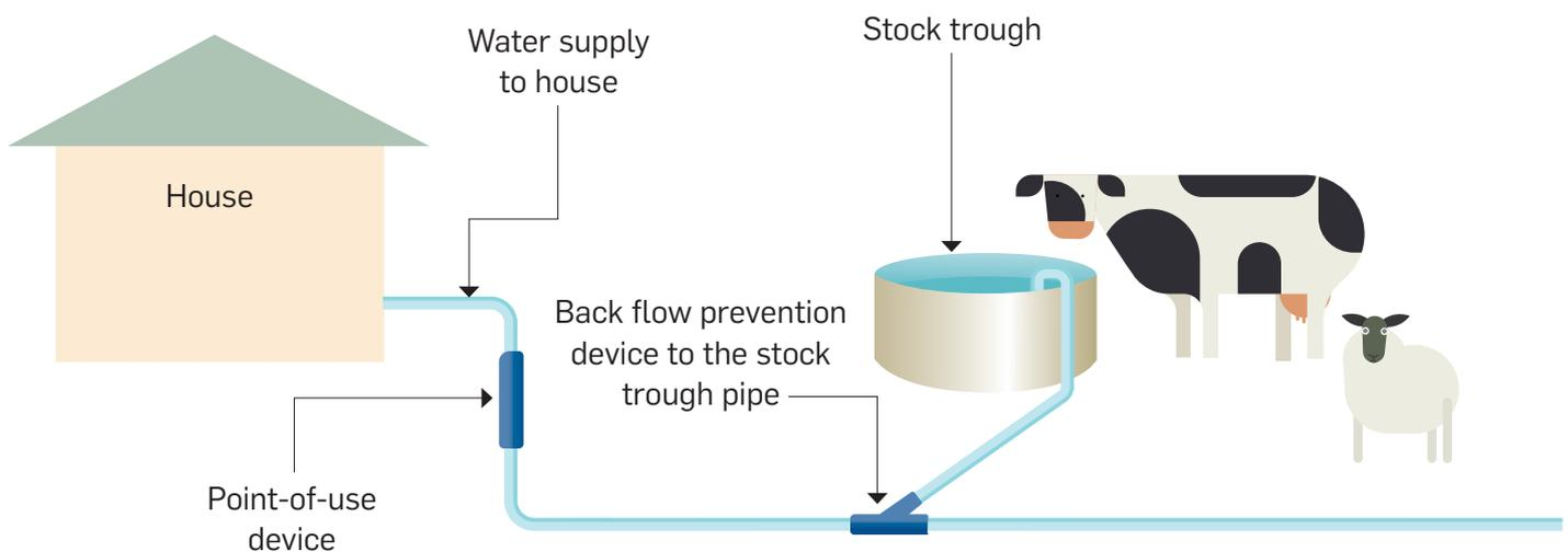
An alternative is to treat water for drinking and cooking purposes only. For this, a bench-top or under-sink point-of-use device can be used, or water can be boiled. However, it must be made clear that water from the other taps is unsuitable for drinking.
