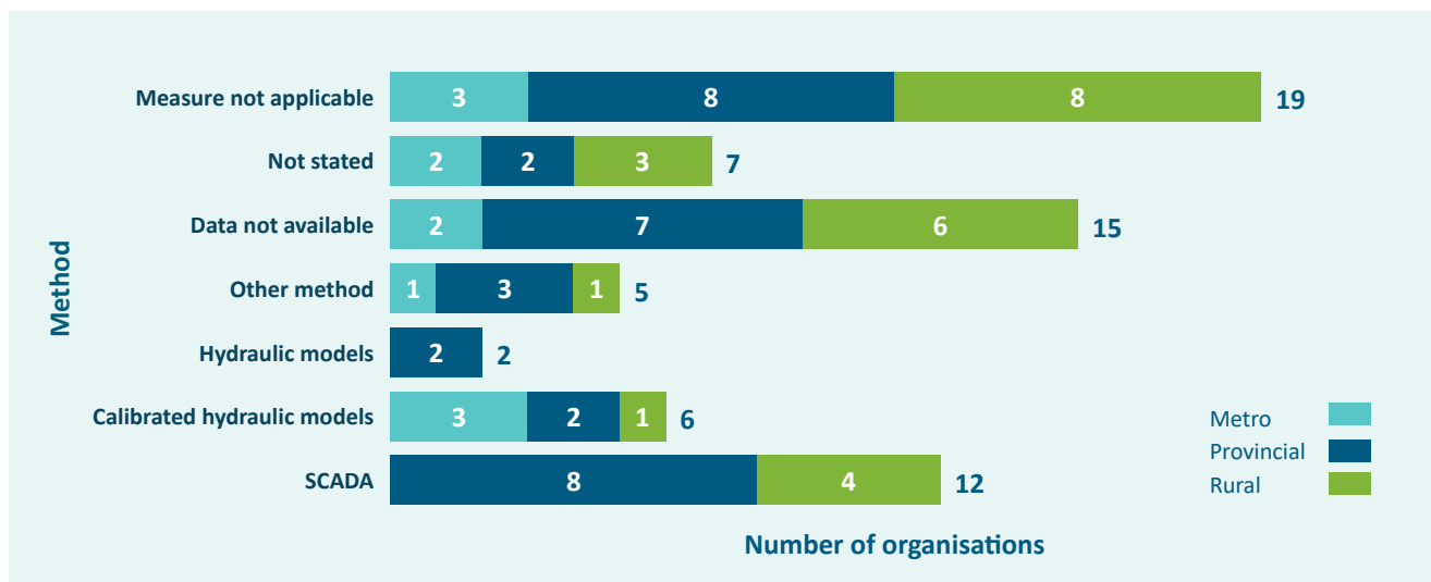
Figure 16: Wastewater overflows by monitoring and calculation method
